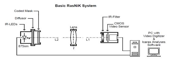
The relative position in X and Y direction is measured along the line mask, optical center of the lens and the CMOS sensor. Also (relative) rotation of the mask or the sensor can be measured. By calculating the actual image spot size and comparing this with the mask spot size, the position of the lens along the Z-axis can be calculated.
