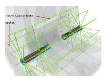
The alignment is not influenced by deformation of RR (sag, spoke load), temperature of individual RR and spoke wheel
