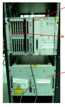
VME crate (ZEUS - Oxford set up ) with new installation of LynxOS 3.01 system, readout cards for sensors pieces of code for software, Box with laser diodes
