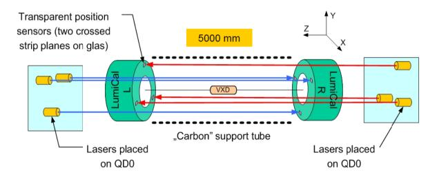
The measurements of the relative distances to QD0 in X,Y and Z directions
