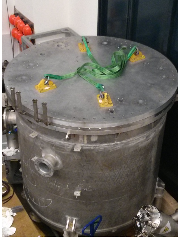
Figure 14: Cryostat that will host the for Mini-ArgonCube detector in Bern.
