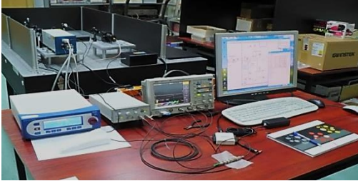
Figure 8. The experimental setup of a single laser FSI system.
