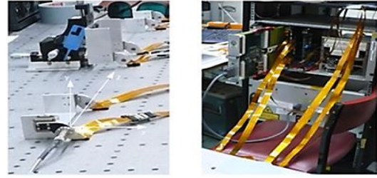
Figure 3. Left: A demonstration prototype; Right: Cards of readout system inside the VME crate.
