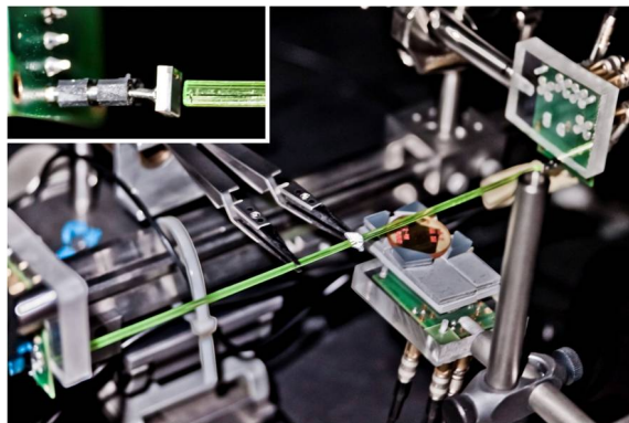
Figure 2. Pictures of the experimental setup used to measure the light output and the light attenuation of the LuAG crystals and fibers.
