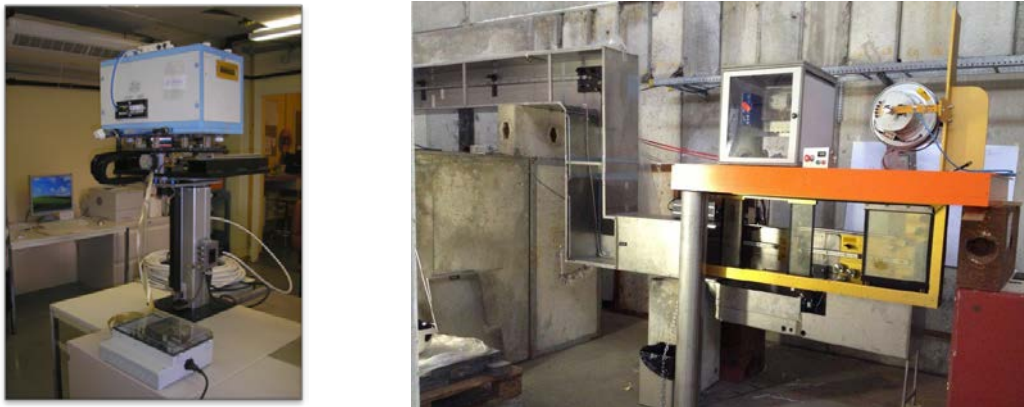
Figure 3: Prototype of a table for proton irradiation equipped with a thermostated irradiation box (left). Loading station of the IRRAD shuttle with its motorization system (picture taken during installation).
