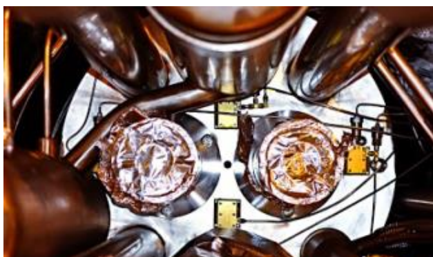
Figure 4: Prototypes of cryogenic BLM installed on the front face of an LHC MQ cold mass.
