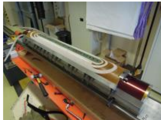
Figure 3: MQXF dummy coil wound at CERN.
