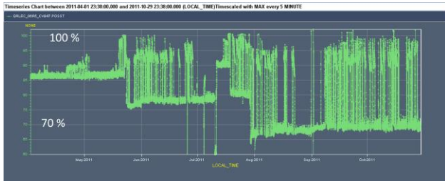
Fig. 12: valve opening for standalone Q6R5 during the 2011 run (April 1 st to October 29 th 2011).
