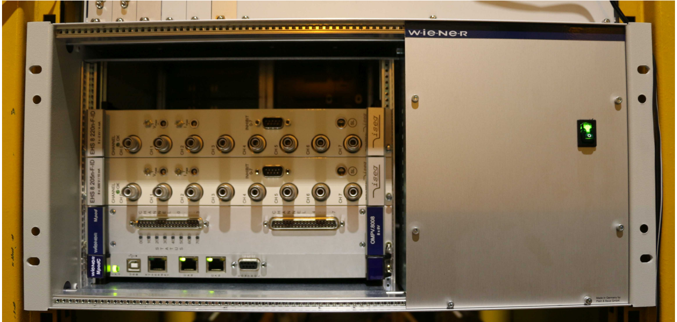
Figure 11: MPod crate with 1 LV and 2 HV modules
