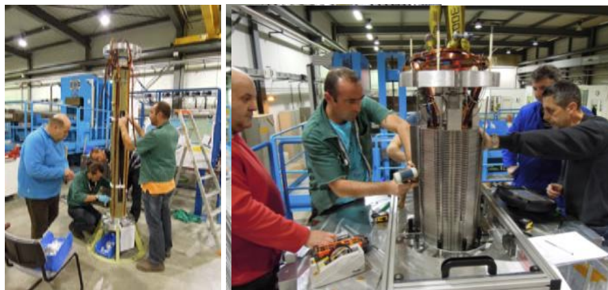
Fig. 3 MQXC assembly: coils around the mandrel (left), the collars around the coils, ground insulation and coil protection sheet (centre) and horizontal collaring (right).
