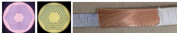
Figure 2: RRP150/169 and RRP108/127 strands and 40-strand cable with a thin stainless steel core.
