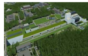
Fig 1. MYRRHA Layout: injector building to the left, the long straight for acceleration and the reactor building to the right. Image Credit: MYRRHA - SCK CEN
