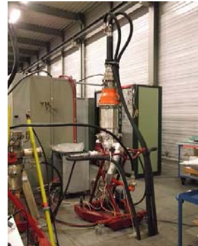
Fig 2. 400 MHz Tetrode Amplifier. Image Credit: Eric Montesinos (CERN)
