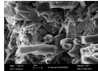
Fig 2. Close up of Molybdenum Graphite sample at nanometre scale. Image Credit: CERN
