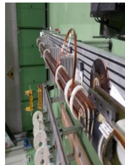
Fig.1. One curved dipole coil of the CRISP project after curing and impregnation of the coil ends. Image Credit: Pasquale Fabbriatore (INFN)
