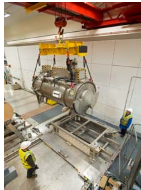
Fig 2. MICE Spectrometer Solenoid Magnet being installed to the beam-line. Image Credit: Stephen Kill (RAL)
