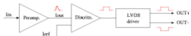
Figure 1: CARIOCA front-end block diagram. Each channel consists of a preamplifier, a three-stage discriminator with an external reference and a LVDS driver.
