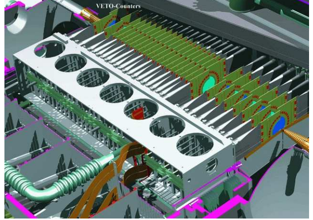
Figure 2: Layout of the Vertex tank with indicated the 2 planes of VETO detectors.
