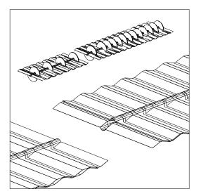
Al box acts as wake field suppressor corrugation needed for upper-lower overlap minimise multiple scattering choice: "toblerone" design, Al  $250\mu$ m (TP:  $100\mu$ m)
