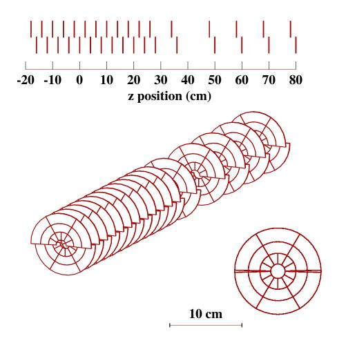
17 disks (stations) of r and  $\phi$  detectors upper-lower halves retract during LHC injection upper-lower overlap for alignment VELO layout (cont'd)
