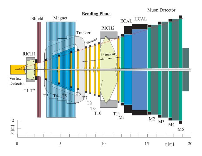
Single-arm spectrometer covering  $\theta$  = 15 mrad to 300 mrad ( $\eta$  = 1.88 to 4.89) Main features: VErtex LOcator (VELO) — vertex detector usual complement of tracking chambers, RICH,
