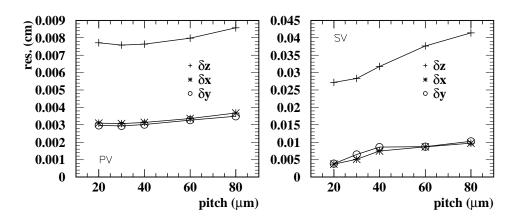
$\rightarrow$  strip pitch important for SV resolution choice: 20/30/40  $\mu{\rm m}$  for r detectors (backup as TP: 40/60/80  $\mu{\rm m}$ )
