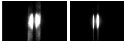
Figure 9. Target images using 0.5 mm target aperture and 2 mm (left), and 1 mm mask aperture (right)
