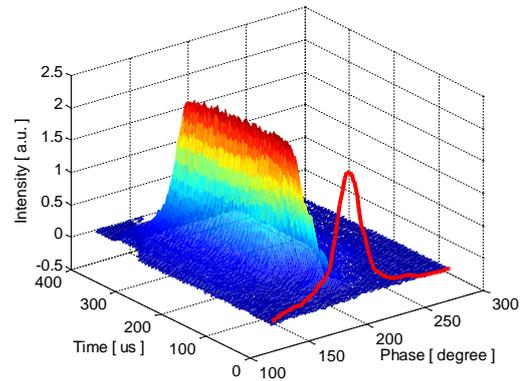
Figure 6: Typical longitudinal distribution acquired by the BSM when the three MEBT bunches are phase tuned.
