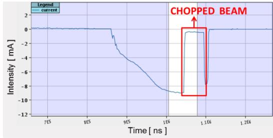
Figure 2: Typical BCT acquisition of the chopped beam.
