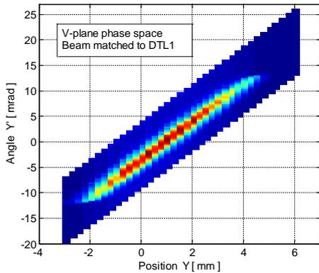
Figure 5: Typical vertical transverse phase space of the 3 MeV H<sup>-</sup> beam when matched to DTL1 tank.
