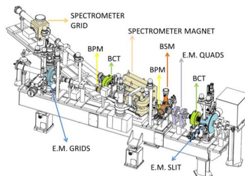
Figure 1: The 3MeV movable diagnostic test bench.
