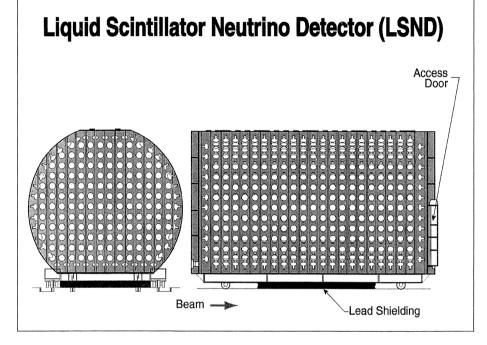
(Above) Schematic of the LSND detector at LAMPF, Los Alamos, designed to search for neutrino oscillations with high sensitivity and to measure the strange quark contribution to the proton spin in neutrino-proton elastic scattering. The tank, approximately 6m in diameter and 9m long, is covered by 1220 8" phototubes and will be filled with 200 t of dilute liquid scintillator (see front cover).
