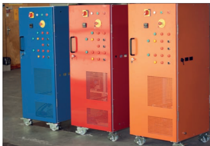
Fig. 5. TRACI prototypes for multipurpose \text{CO}_2 cooling under construction at CERN. (Image credit: Kamil Cichy.)
