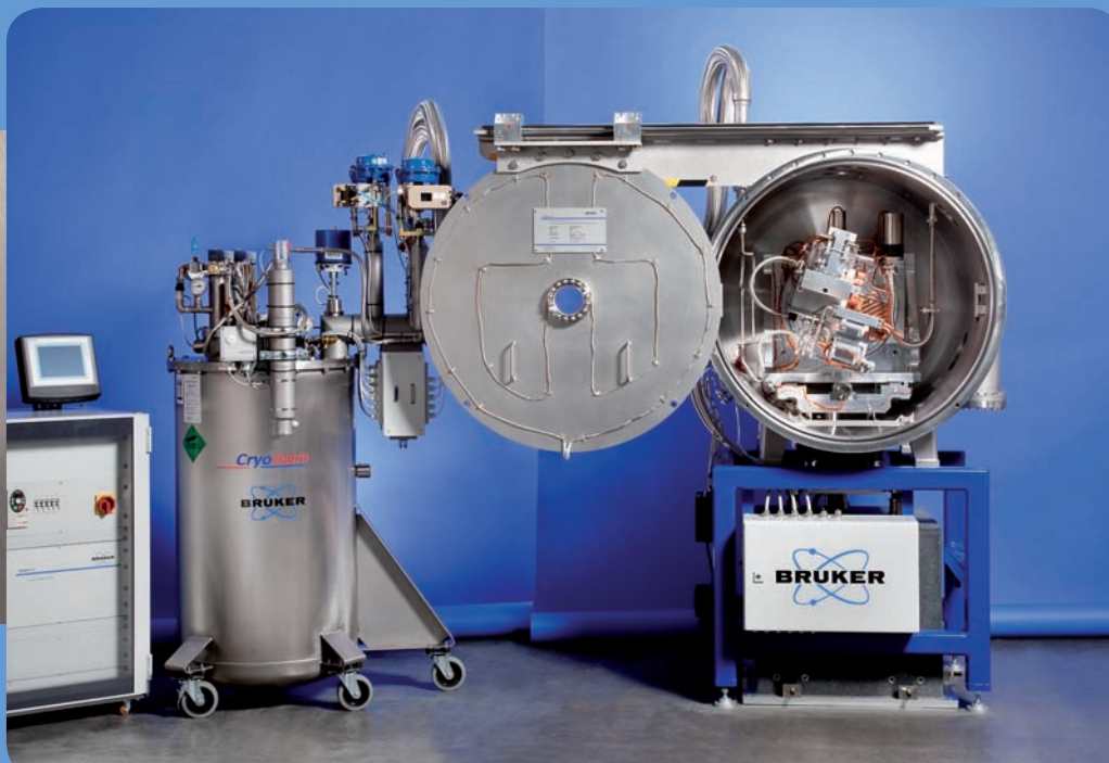
Double Crystal Monochromator with Cryo Cooler
