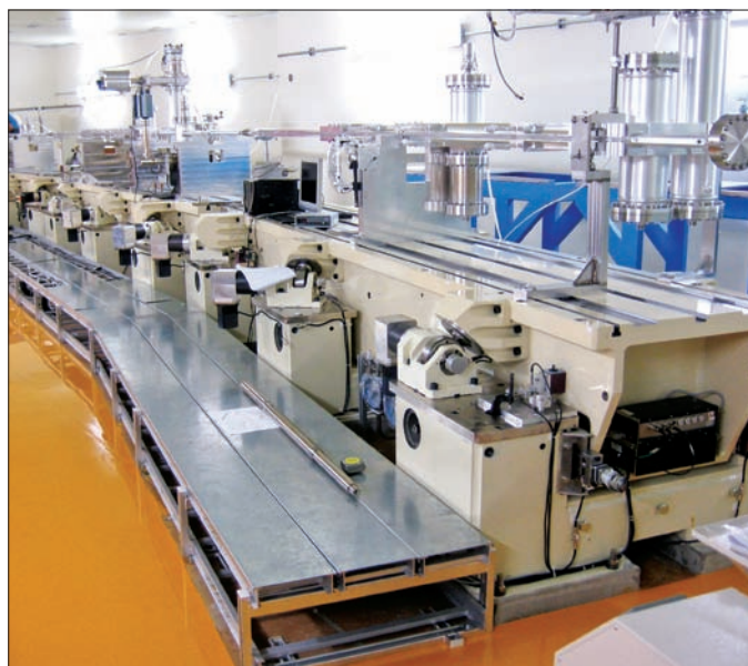
A complete mock-up of 1/24 of the storage ring was built for tests.
