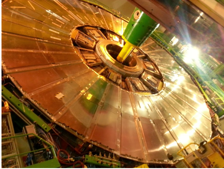
Figure 2. One of the two CMS endcap disks fully instrumented with RPC detectors.
