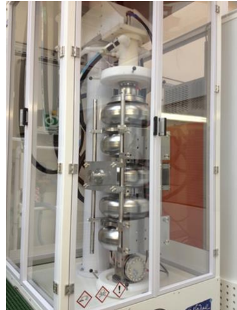
Figure 39: 704 MHz \beta=1 5-cell cavity installed in the vertical electro-polishing set-up (courtesy CEA)
