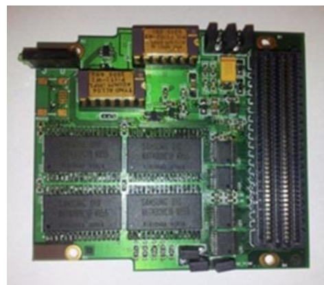
Figure 44: \mu TCA RadFETs dosimeters for FLASH, (courtesy DESY)
