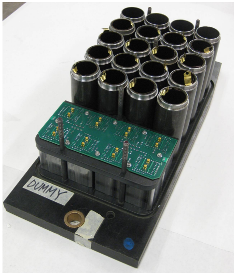
Figure 9. “Plate 2”; part of readout box with R7525s and R7600s for CMS HF.
