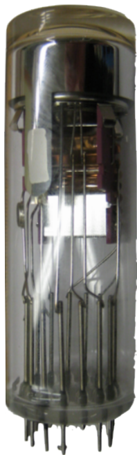
Figure 2. Hamamatsu R7525 – The original HF PMT
