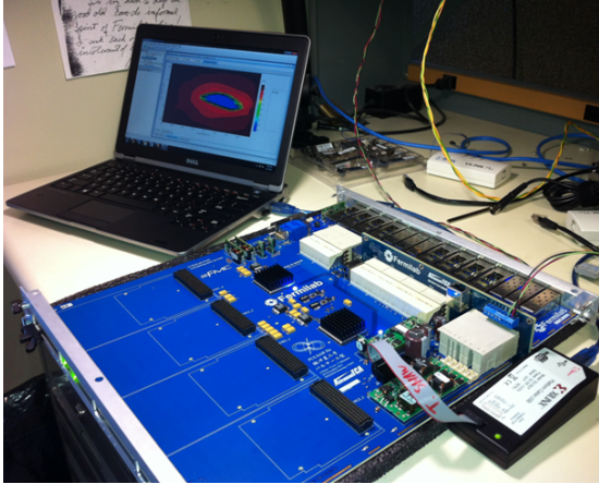
Fig. 9. The mini backplane powers the Pulsar IIA board on the bench top. A laptop and 48VDC power supply is all that is required to power up and test the Pulsar IIA board and RTM.
