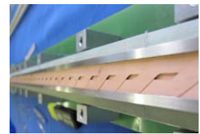
A Roebel cable prototype, inserted in a sample holder and ready for test at low temperature and high field in the CERN FRESCA test facility. Image credit: J. Fleiter, CERN
