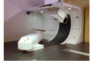
Spot scanning gantry ( Gantry 2 ), which was designed specifically to enable treatment of moving tumours with scanned beams. Image credit: PSI.
