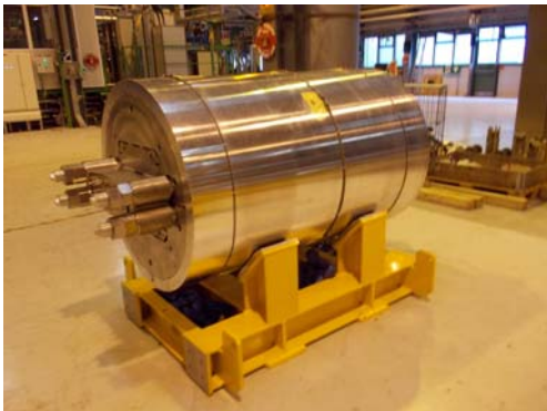
Fig. 5. FRESCA2 structure completely assembled
