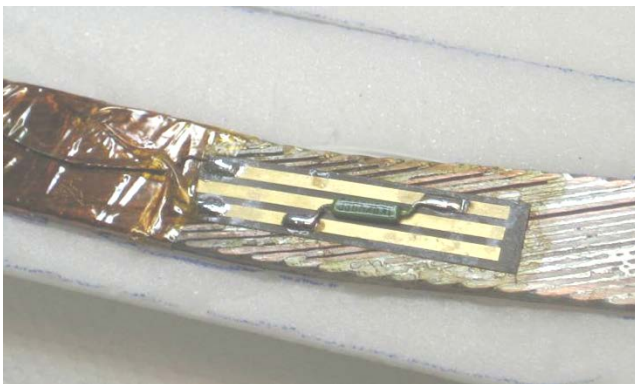
Fig. 4: CCS sensor T2, mounted on MQXC superconducting cable with use of thermal pad.
