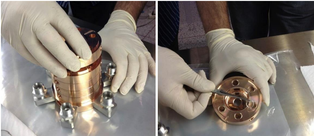
Fig. 4: Preparation of the cells. Stacking the cells (left), inserting alloy rings for brazing (right).
