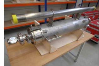
XFEL series cavity during incoming inspection at DESY. Image credit: DESY.
