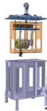
Fig 1: Top-loading of the cryostat with a double spoke cavity. Image credit: TIARA.
