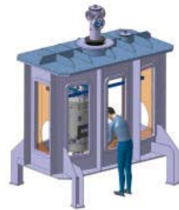
Fig 2: Cryostat integrating a quarter-wave resonator. Image credit: TIARA.
