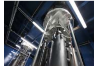
Vertical test inserts equipped with XFEL superconducting accelerator series cavities. Image credit: DESY.
