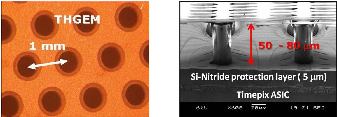
**Fig. 4:** (left) Photo of the Thick GEM (THGEM) multiplier; (right) photo of the “InGrid” detector with  $\sim 5 \mu\text{m}$  silicon-nitride protection layer.
