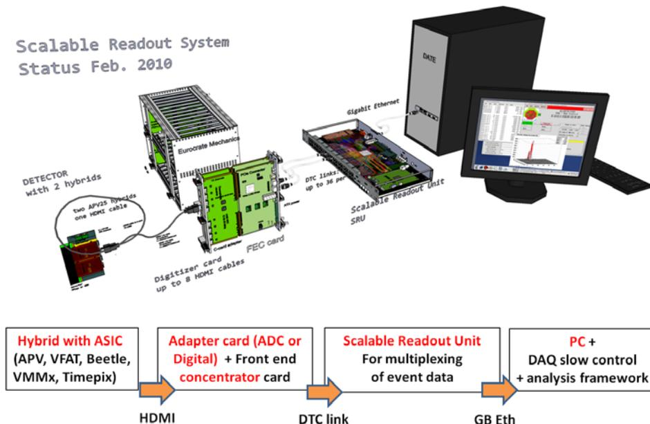
**Fig. 7.** Sketch of the SRS readout architecture, consisting of front-end ASIC on hybrid, a chip-link implemented via HDMI cables, an adapter to a common FEC card and a direct Ethernet connection to an Online PC. Medium-sized systems with several FEC cards require an Ethernet switch and large systems require an Scalable Readout Unit (SRU).
