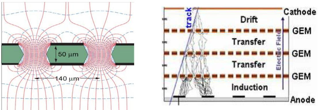
**Fig. 2:** (left) Schematic view and typical dimensions of the hole structure in the GEM amplification cell. Electric field lines (solid) and equipotentials (dashed) are shown; (right) schematic view of the triple-GEM detector.
