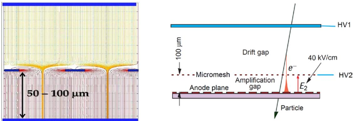
**Fig. 3:** (left) Electric field lines in Micromegas; (right) schematic drawing of the Micromegas detector.
