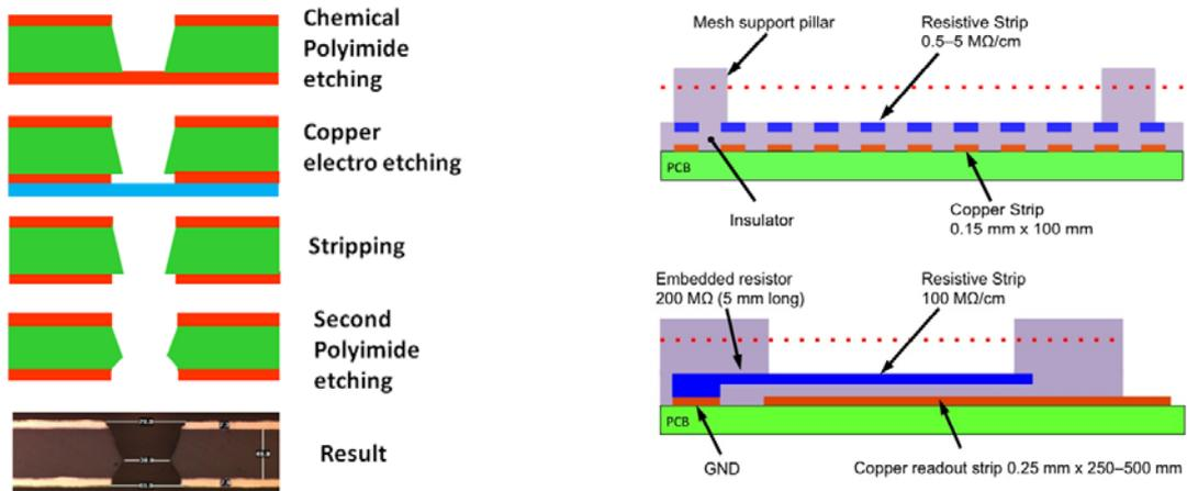
**Fig. 6:** (left) sketch of the single mask GEM technology; (right) sketch of the resistive Micromegas principle, illustrating the resistive protection scheme.
