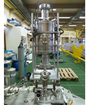
Fig 1: 4-rod crab cavity for HL-LHC. Image credit: ULANC.
