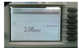
Fig 2: Power meter display showing peak pulsed power. Image credit: TIARA/MICE.
