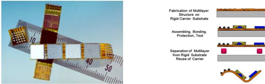
Figure 8. Medical flexible polyimide circuit (left) and fabrication method (right).
