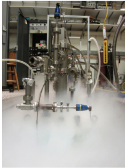
FIG. 20: A photograph of the top of the Project 8 prototype magnet during cool down.
