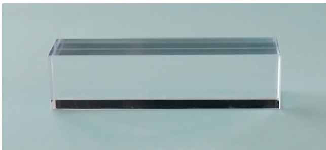
Fig. 1. One of the tested LYSO samples, showing excellent mechanical processing and optical surface treatment.
