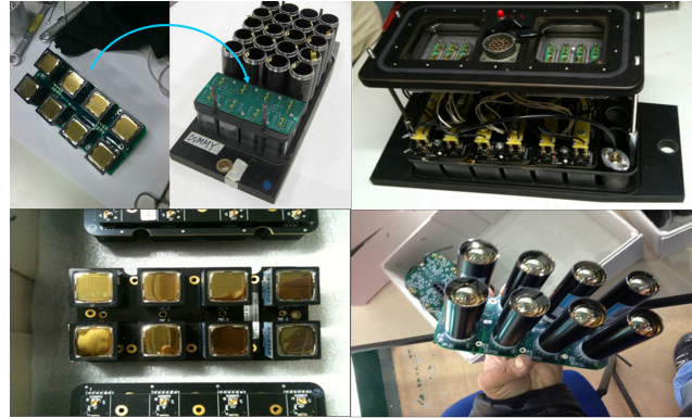
Fig. 3. A picture of the modified robox for the slice test during 2011 and 2012 runs (top left); robox modified for the 4-anode PMTs (top right); 4-anode PMTs installed in their baseboards (bottom left); old single anode PMTs removed from the detector (bottom right).
