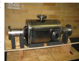
LHC 4-rod Crab Cavity Fabricated. Image credit: Niowave Inc (USA)
