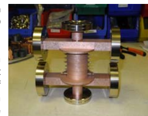
CLIC 'Undamped' Crab Cavity Fabricated. Image credit: Shakespeare Engineering Ltd (UK)
