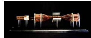
Maquette of High Temperature Superconducting Link of the type needed at LHC Point 7. Image credits: CERN
