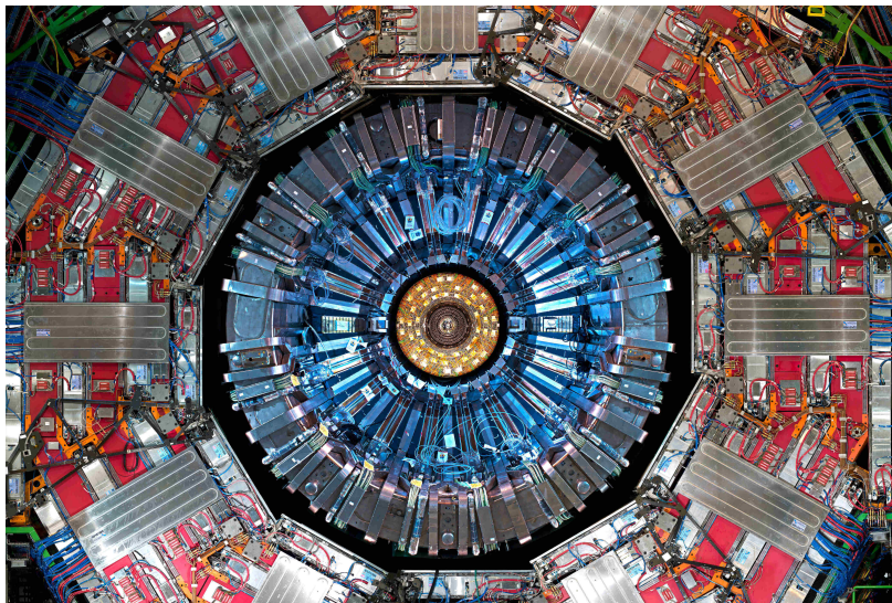
Figure 3.3. The transverse view of the CMS detector during assembly.
