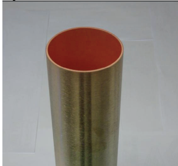
Figure 6: Copper coated RHIC tube sample.
