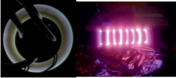
Figure 8: Photo of argon plasma between magnetron surface and tube (left); power, cooling, and instrumentation feed visible; plasma discharge and deposition are azimuthally uniform. But axially discharge is non-uniform (right).
