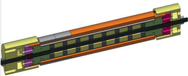
Figure 9: Drawing of bi-metal titanium-copper magnetron.
