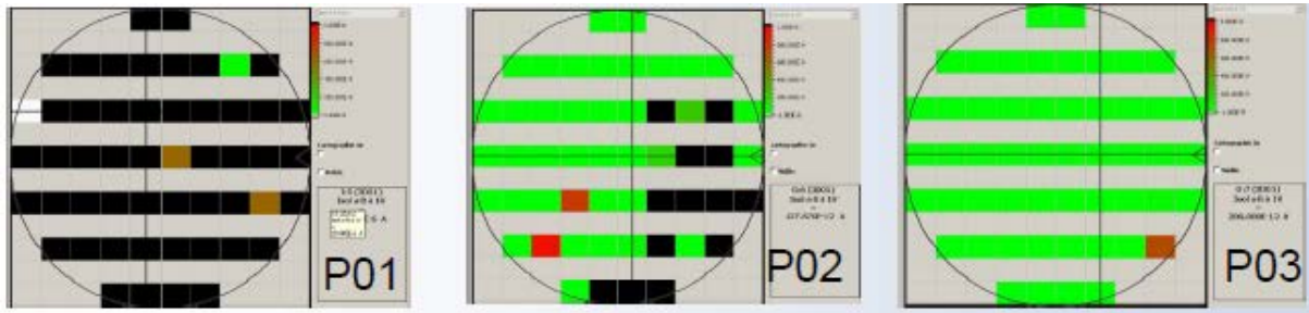
Fig. 1: Insulation between TSVs and bulk of the various sub-batches. While the first batch showed very low yield (chip marked black) the consecutive batches showed large improvements up to almost no defects.
