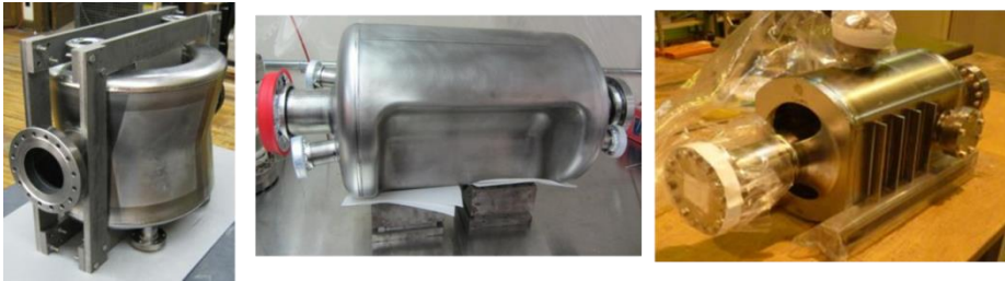
Figure 22: Prototypes of the three crab cavity designs fabricated in bulk Niobium (Courtesy Brookhaven National Lab, Old Dominion University, Lancaster University and Niowave Inc).
