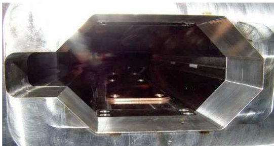
Fig. 5: Installed electrode in the dipole vacuum chamber.
