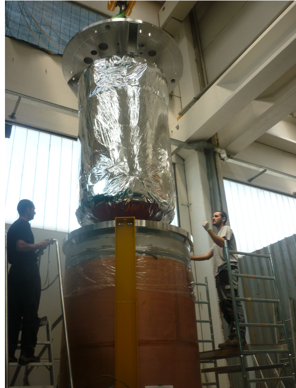
Figure 12: Insertion of the IVC into the 300 K vessel before the cold tests. The 4 K vessel and plate is wrapped with superinsulation.
