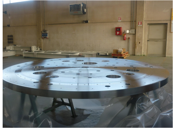
Figure 8: The 300 K plate after cleaning at the production site.
