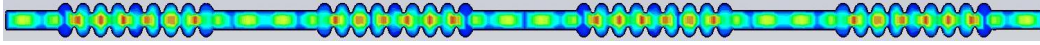
Figure 2.15: The electric field distribution of the strongest coupled cavity mode from the first dipole band (frequency: 4.8076 GHz, R/Q : 125.762 \Omega/\text{cm}^2 per module). Electric (EE) boundary conditions were used in the simulation.
