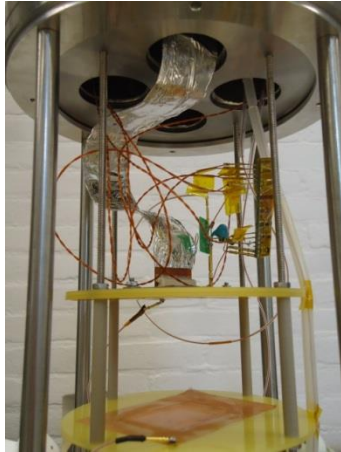
Figure 8: Picture of the TPC mounted to the top flange of the vessel with data cable and preamplifier.
