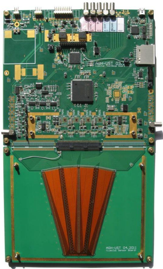
Figure 7 A sensor plane assembled with front-end and ADC
