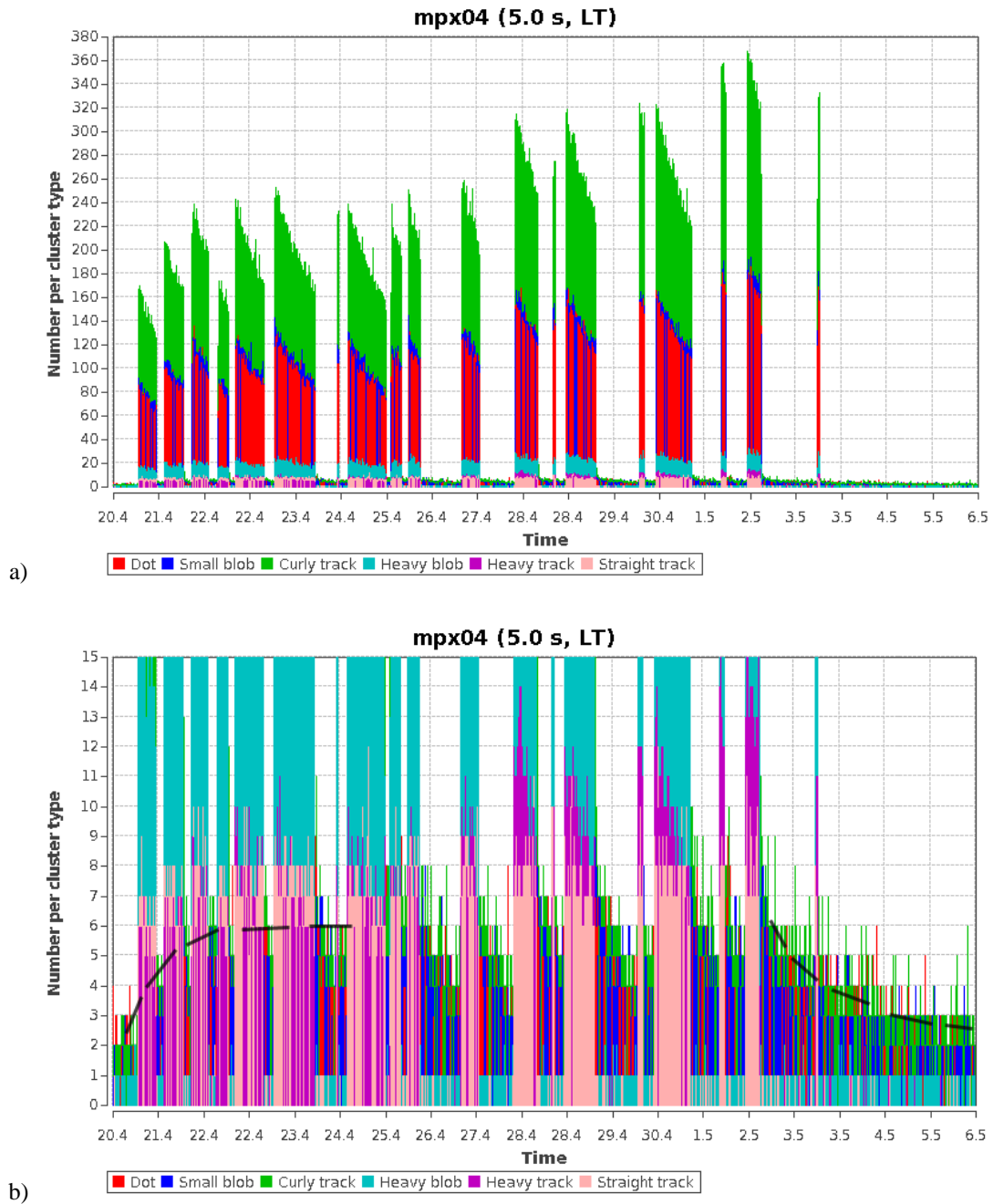
Figure 24. a) Cluster counts of different cluster types as measured with MPX04 between 20 th April and 6 th May 2011. b) Detail of the previous figure. The exponential increase of induced activity of the long decay component due to the first fills and decrease after the last fills are clearly visible (highlighted by dashed black curves).
