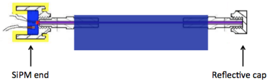
Figure 33: Single-ended readout with SiPM of fiber embedded in a plastic scintillator bar.
