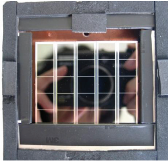
Fig. 3: Photograph of the detection module of the small HICAM prototype. The whole active area is 5 cm x 6 cm.
