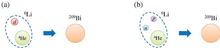
Fig. 1: (Color online) Schematic picture of three- and four-body systems. (a) represents d+{}^4\text{He}+{}^{209}\text{Bi} three-body model, and (b) represents p+n+{}^4\text{He}+{}^{209}\text{Bi} four-body model.
