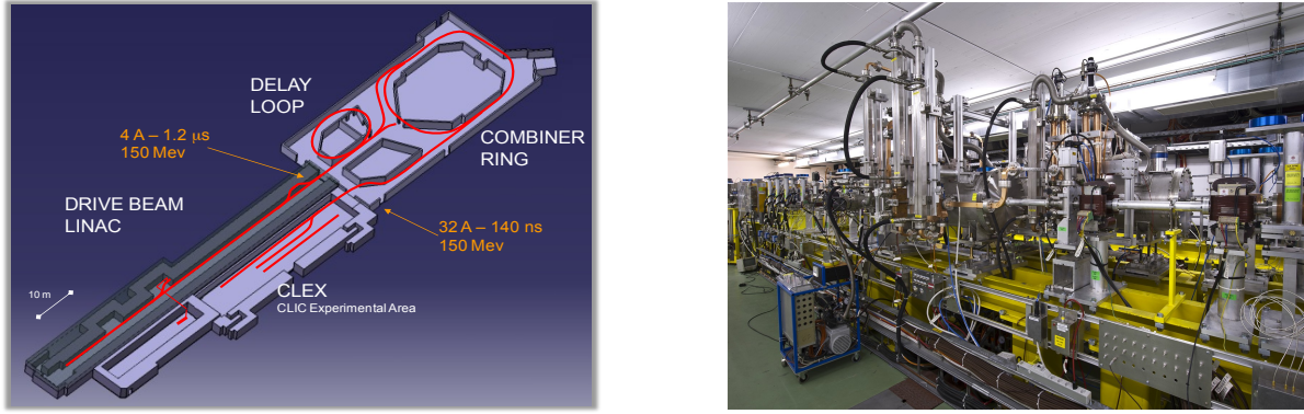
Fig. 3.3: Left: Layout of CTF3. Right: The two-beam test stand in CTF3.
