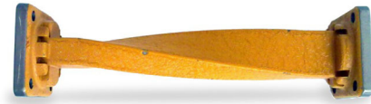
FIG. 6 (color online). Twisted waveguide section (90°). A structure consisting of several straight sections connected by 180° twists is predicted to have a high geometric factor close to C \approx 0.6 in a dipole magnet, while avoiding many engineering challenges of other setups.
