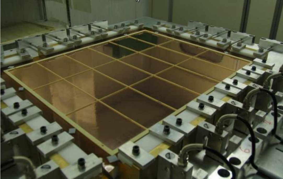
Figure 7. First full scale GEM module prototype during assembling. Three components are visible: the stretched GEM foil; the thin support PERMAGLAS frame with the spacers which form 18 open sectors (their configuration is different respect to the final version presented in figure 2 and 6); the foil stretcher, whose design is derived from [20].
