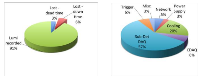
Fig. 5. Overall CMS data taking efficiency in 2011; left chart shows total luminosity recorded by the experiment, right chart provides a breakdown of causes for downtime.
